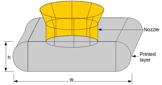
**Fig. 3:** Cross-section of the nozzle and printed layer
