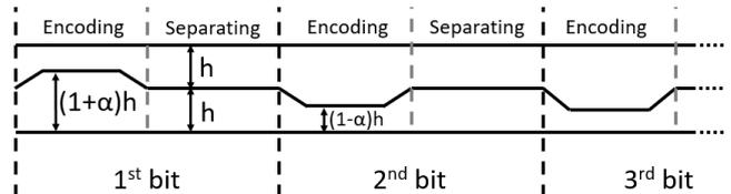
**Fig. 1:** Encoding layer pattern. It corresponds to 2 layers with variable thickness. We can encode a 1 or 0 bit by respectively increasing or decreasing the thickness of the bottom layer in the encoding region. The top layer thickness will be adjusted such that the sum of the thickness of the 2 layers stay equal to  $2h$ . The separating region always keep a thickness  $h$ .
