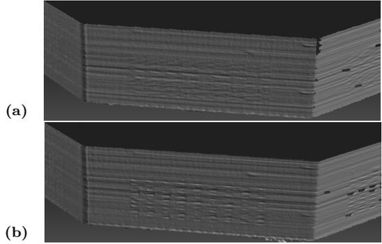
**Fig. 4:** 64 bits watermarked object scanned by 'HP 3D structured light scanner pro S3' (a) with adjustment of the plasting extrusion to the layer thickness (b) without adjustment
