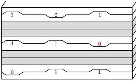
**Fig. 2:** Example of the watermark pattern Encoding the value "1011" + the parity bits. The digits correspond to the encoded bits, those in red are parity bits. The layers with white background are encoding layers, those in gray are separating layers.
