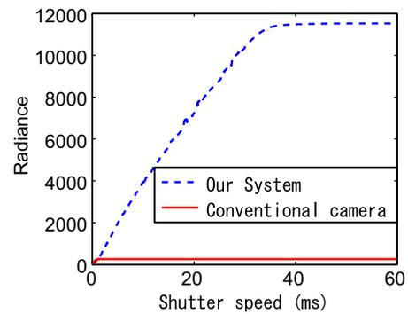
Fig. 8. Comparison of system outputs obtained from Fig. 7. The radiance outputs are calculated from Eq. (2).
