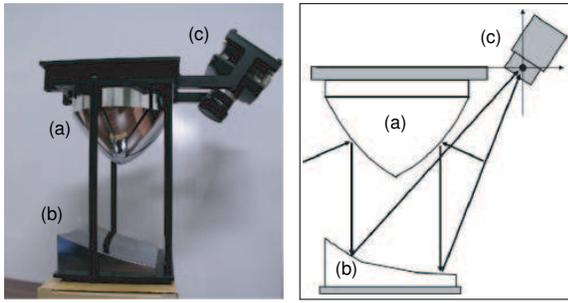
Fig. 2. Prototype of the HBP mirror system and its geometry model. A ray from a point in a scene is reflected by the HBP mirror(a) and reflected again by a parabolic mirror(b) to concentrate on a perspective camera(c).
