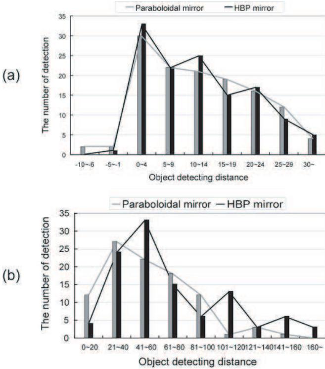
Fig. 16. Histograms of the detection distances. (a) detections of objects on the alleys. (b) detections of objects on the main route.
