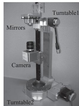
Fig. 4. Experimental calibration system with two turntables.
