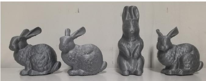
Fig. 13: Real print of watermarked models. From left to right : bunny 8 bits, reprint 90° of bunny 8 bits, rabbit 8 bits, bunny 16 bits. For the second bunny, we used the first bunny, scanned it, then printed the scanned model with a 90° angle, some degradations are visible because we printed it on the side, and the surface was on contact to the support material.
