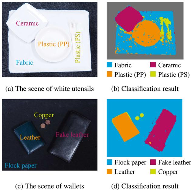
Figure 8: Material segmentation results. (a) All utensils are white hence it is difficult to classify only with an RGB image. (b) The result of our material classification. Although there are some estimation error because of the pixel-wise process and only one depth variation, the scene is much interpretable than the RGB image. (c) Wallets made of genuine and fake leather and copper coins are placed in the scene. (d) Material segmentation result.
