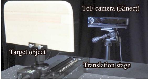
Figure 3: Experimental setup. We use Kinect as a ToF camera, and the target object is placed on a linear translation stage.
