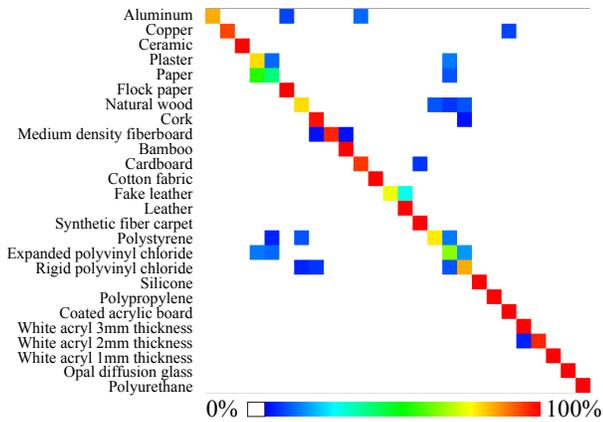
Figure 5: Confusion matrix. Red indicates the higher value and it appears on the diagonal. Overall accuracy is 90.5%.
