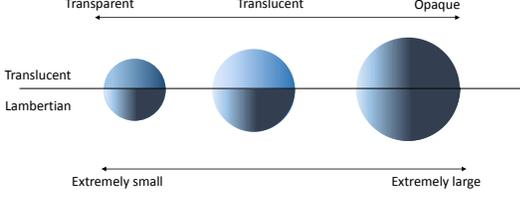
Figure 2. How surface curvature affect translucency
