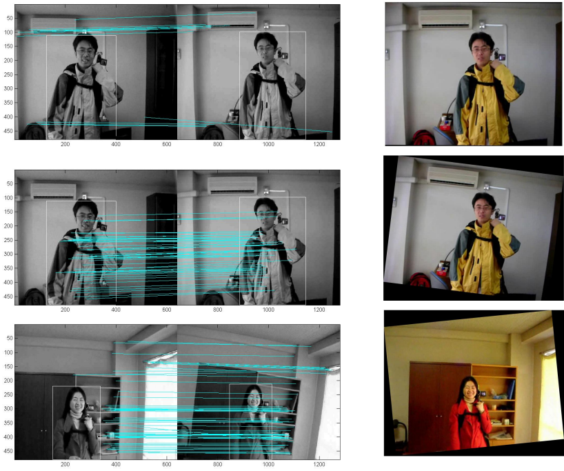
Fig. 6. One set of data for transformation computation (A and B) in calibration stage. Left column: Up) Point matches in background region of video2; Middle) Point matches in foreground region of video2; Down) Point matches in background region of video1. Right column: Up) stabilization result using background region in video2. Middle) stabilization result using foreground region in video2. Down) Stabilization result using background region in video1.
