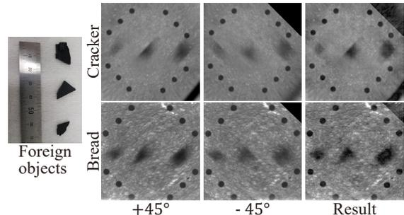
Figure 8. Results with real food, showing that our proposed method worked successfully in the prototype system and high-frequency detail was obtained.
