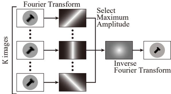
Figure 4. Integration in the Fourier domain. Applying Fourier transform to the observed images,  $K$  images are obtained. For each frequency in the Fourier-transformed image, the component with the maximum amplitude among the  $K$  images is selected and integrated into a single image. The integrated clear image is recovered by applying inverse Fourier transform.
