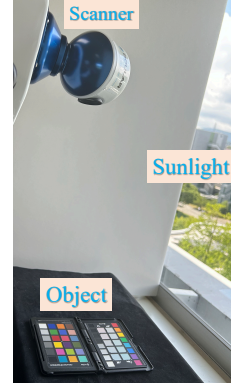
Fig. 2: Experimental setup: The object is a colour chart of ColorChecker Passport (X-rite, Inc) under uncontrollable illumination near a window.
