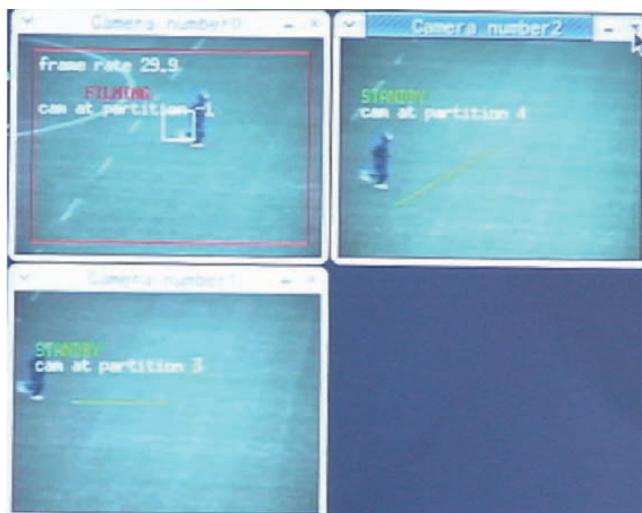
Figure 9 Tracking result 1 using 3 cameras; while the monitoring camera is filming the object, each of the stand-by cameras takes a position and waits for the target
