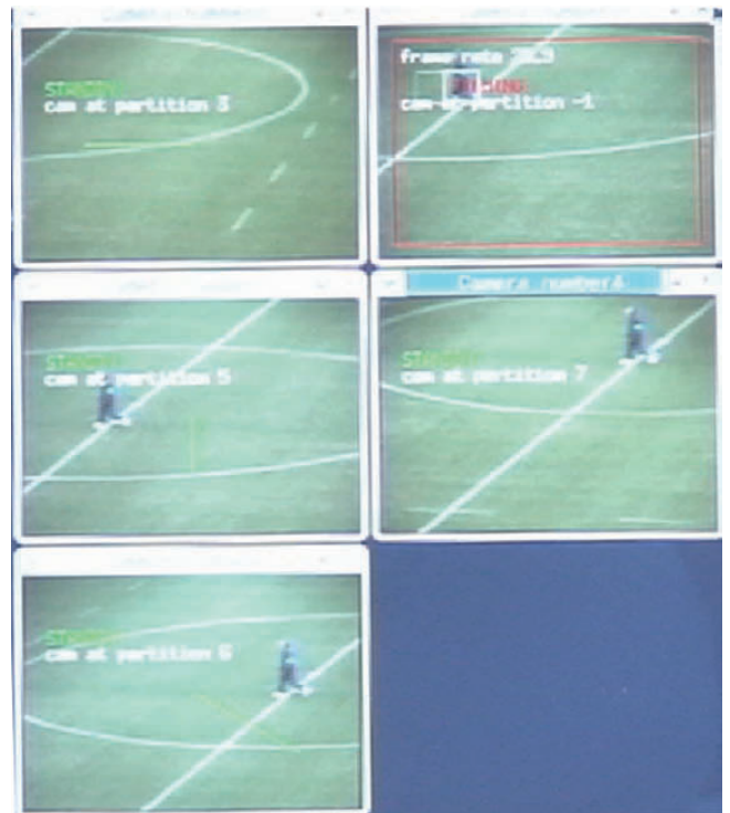
Figure 12 Tracking result 2 using 5 cameras; while the monitoring camera is filming the object, each of the stand-by cameras takes a position and waits for the target
