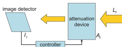
Fig. 1. Incident light is adaptively controlled by changing attenuation ratios based on incident radiance.
