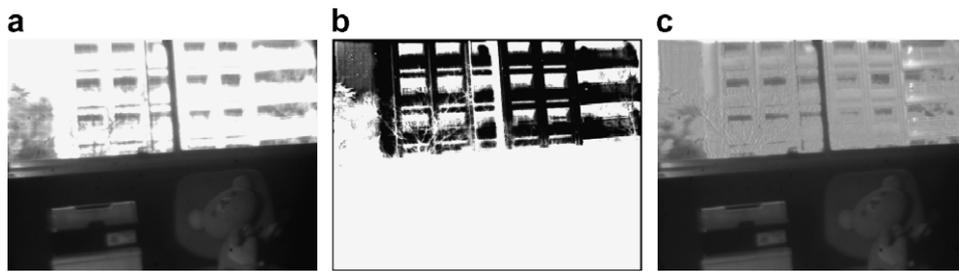
Fig. 9. An outdoor scene taken through a window. (a) Captured image with uniform highest attenuation (initial scene), (b) controlled attenuation for the scene, (c) captured image after attenuation control. We captured a window from the inside as an example of a scene that includes drastic lighting changes.
