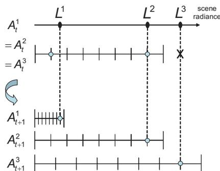
Fig. 4. The concept of adaptive attenuation control. Attenuation control enables the image detector to accept various ranges of radiance with the least quantization errors.
