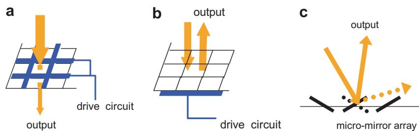
Fig. 2. Simple models of light controlling devices: (a) transmissive liquid crystals, (b) reflective liquid crystals and (c) DMDs. The properties of each device, as used in our system, are compared in Table 1.
