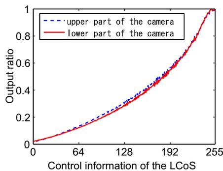
Fig. 6. The output ratio of the LCoS. LCoS attenuation response for 8 bit control. The response is measured at the upper and lower parts of the camera coordinates. The vertical axis represents the attenuation ratio of the LCoS. The horizontal axis represents the depth of attenuation control. A depth of 255 implies the highest attenuation, similar to the color representation used in many image formats.
