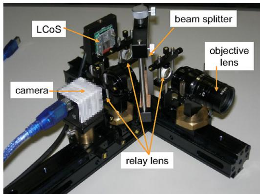
Fig. 5. Implementation of the prototype system. The system consists of a monochrome camera, reflective liquid crystal, and lenses used as relay and objective lenses. The system is covered by a jig for capturing.
