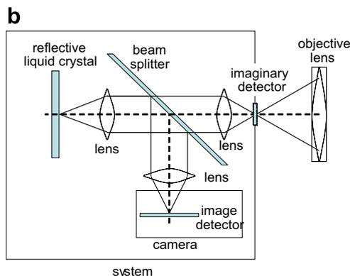
Fig. 3. Imaging system using reflective liquid crystal: (a) basic composition, (b) advanced system with relay-lenses. The incident light is first focused onto the liquid crystal plane. The reflected light is refocused onto the image detector.
