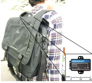
Figure 3. Our experimental sensor system consisted of an inertial sensor, fixed under the handle, connected to a small computer inside the back-bag.
