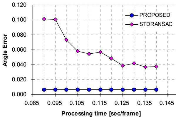
Fig.13. Outdoor environment: estimation errors with different processing time. Translation is 30[cm] and angular velocities are  $\omega_{\theta} = 10$  [deg/frame],  $\omega_{\phi} = 5$  [deg/frame] and  $\omega_{\psi} = 0$ .
