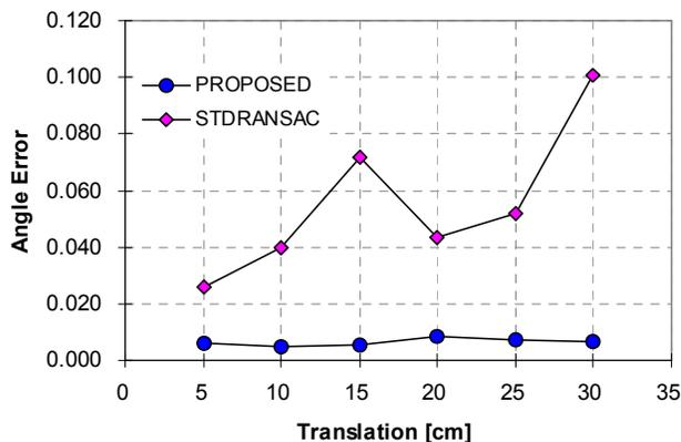
Fig.11. Outdoor environment: estimation errors with different camera translation. Processing time is 0.1 [sec/frame] and angular velocities  $\omega_{\theta} = 10$  [deg/frame],  $\omega_{\phi} = 5$  [deg/frame] and  $\omega_{\psi} = 0$ .
