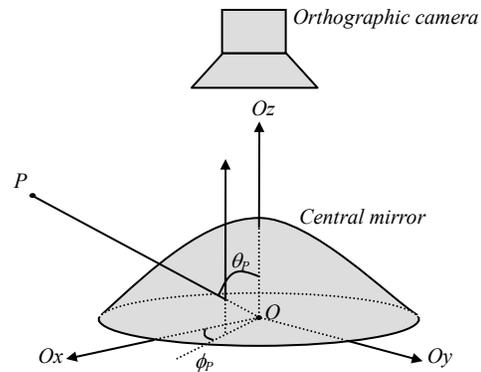
Fig. 2. Camera coordinate system.
