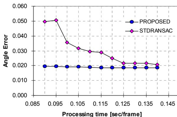
Fig. 9. Indoor environment: estimation errors with different processing time. Translation is 25[cm] and angular velocities are  $\omega_{\theta} = 10$  [deg/frame],  $\omega_{\phi} = 5$  [deg/frame] and  $\omega_{\psi} = 0$ .
