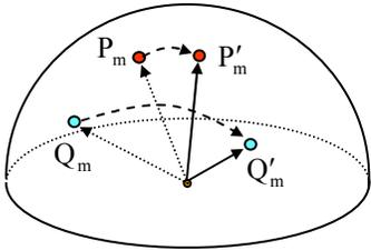
Fig. 3. Estimate rotation from motion of 2 points.
