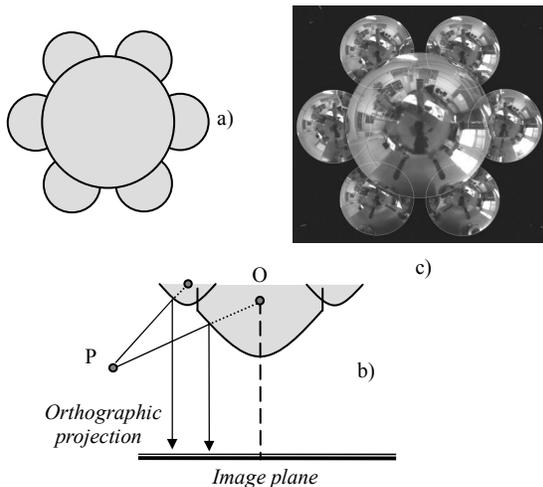
Fig.1. Top view (a), side view (b) of the mirrors and omni-directional image from the compound sensor (c).
