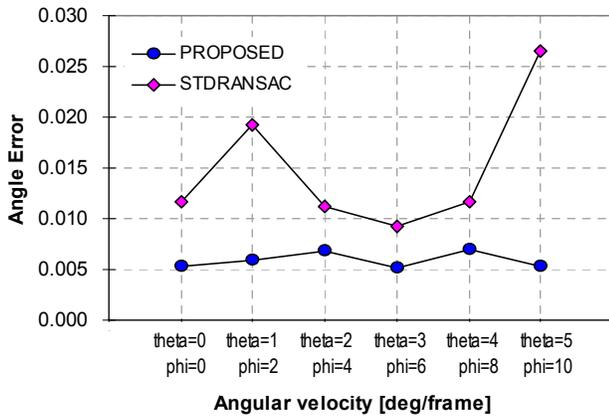
Fig.12. Outdoor environment: estimation errors with different angular velocities. Processing time is 0.1[sec/frame] and translation is 15[cm].
