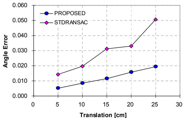
Fig. 7. Indoor environment: estimation errors with different camera translation. Processing time is 0.95 [sec/frame] and angular velocities are  $\omega_{\theta} = 10$  [deg/frame],  $\omega_{\phi} = 5$  [deg/frame] and  $\omega_{\psi} = 0$ .
