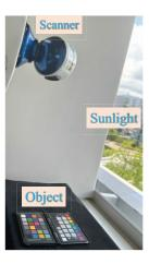
Figure 3: Experimental setup: The object is a colour chart of ColorCheckerPassport (X-rite, Inc) under uncontrollable illumination near a window.
