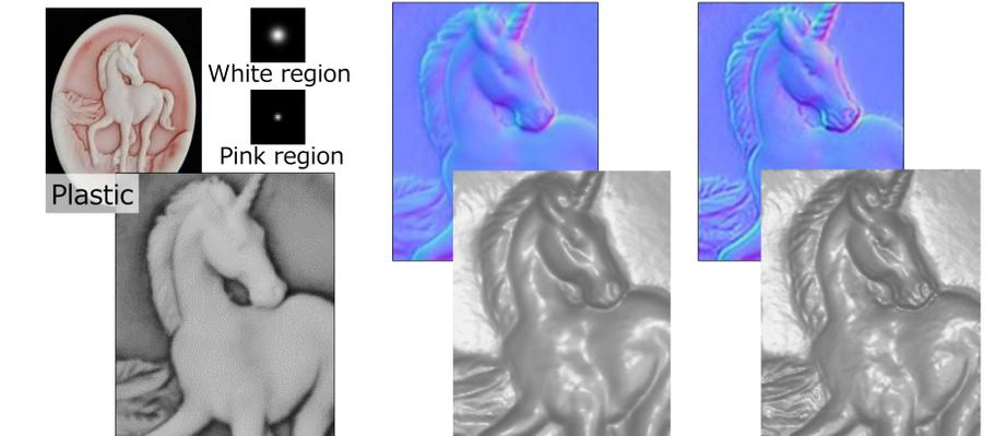
Observed shading image and scattering filter      Lambertian photometric stereo      Our method
