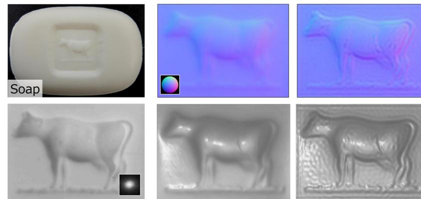
Observed shading image and scattering filter      Lambertian photometric stereo      Our method
